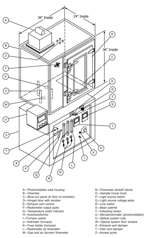
FIG. 1 Smoke Density Chamber Assembly
